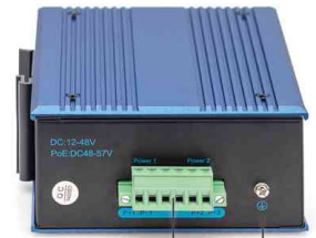
Terminal block Grounding Erdung
